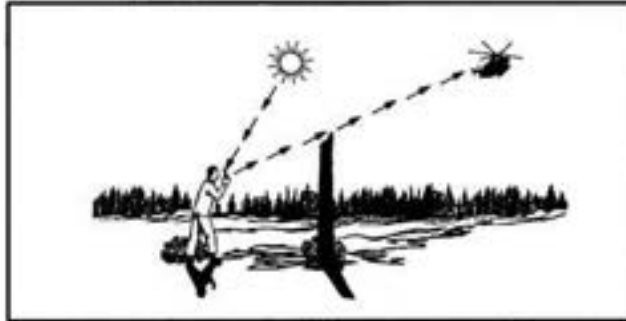
Figure 19-5. Aiming an improvised signal mirror—stationary object.
