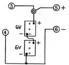
Batteries are wired in series to increase voltage.
