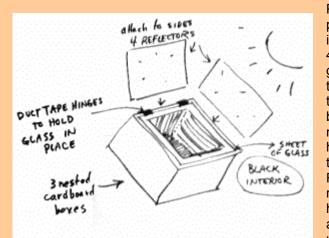
A solar oven design made with cardboard boxes, aluminum foil, and a piece of window glass. Interior of the box is flat black paint.
