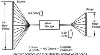
water source quickly accumulates enough water to handle a standard household (Fig. 4).
