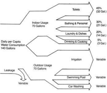
Understanding how water is used helps conservation and gray water system design.
