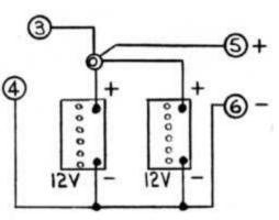
Batteries may be wired in parallel to increase capacity.
